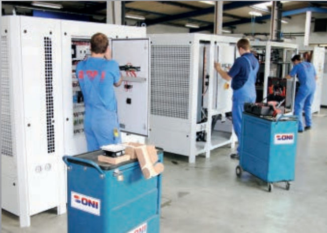
Luftgekühlte Kompakt-Kältemaschine in der Endmontage Air-cooled compact chiller in its final assembly
